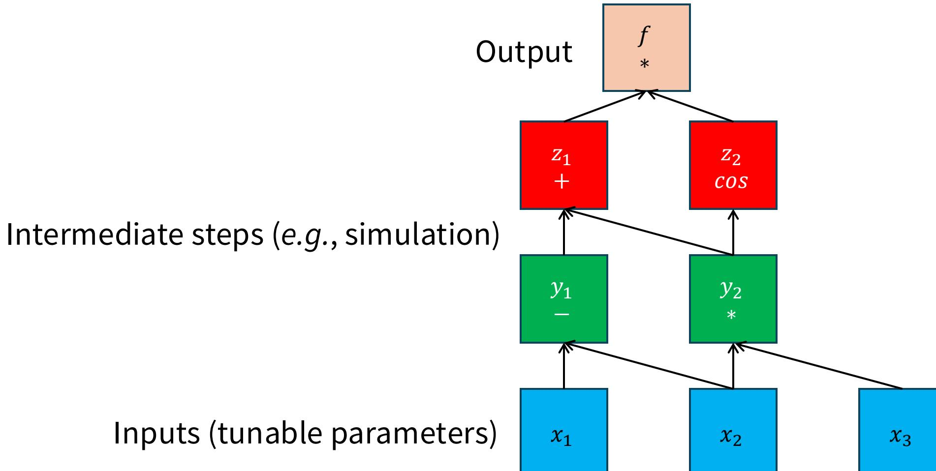
$$f(x_1, x_2, x_3) = \overbrace{(x_1 - x_2 + x_2 x_3)}^{z_1} * \overbrace{(\cos x_2 x_3)}^{z_2}$$
