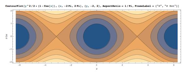
Note that when the energy reaches a critical value, there is a crossing point at  $\theta = \pm \pi$  that the system does not actually achieve in finite time. The crossing point is called a separatrix, which separates the phase space into distinct regions (bound and unbound motion).
